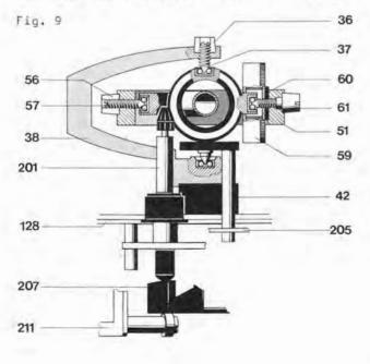
of tonearm and chassis resonance. For this purpose, the inner part weight is matched to the tonearm resonance and thus acts as anti-resonator by means of antiphase vibration. The outer part of the balance weight taking the form of a higher balanced antiresonator prevents transmission of partially occurring chassis resonance to the tonearm. U.
